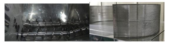
The above left photo is the auger inside the product hopper for conveying product from hopper to pulverizing chamber.
