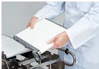
The conveyor unit can be attached or detached from the motor easily, thus facilitating cleaning.
